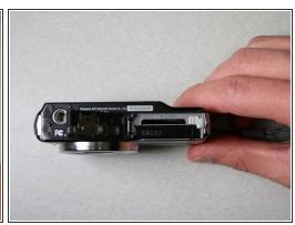
On the bottom of the camera, move the gray switch that has the words "open" and "lock" above it to the open position. The case will open.
