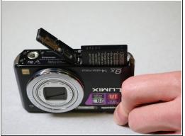
Once the case is open, there will be another switch on the right side of the battery. Push the switch
