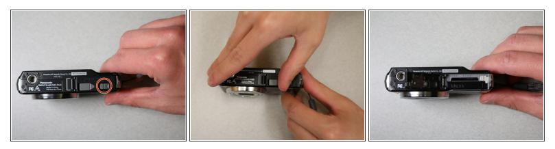
• On the bottom of the camera, move the gray switch that has the words "open" and "lock" above it to the open position. The case will open.
