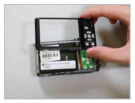
Remove the back panel. This might require some extra force. If you still can't get the panel off, try to use a plastic opening tool.
