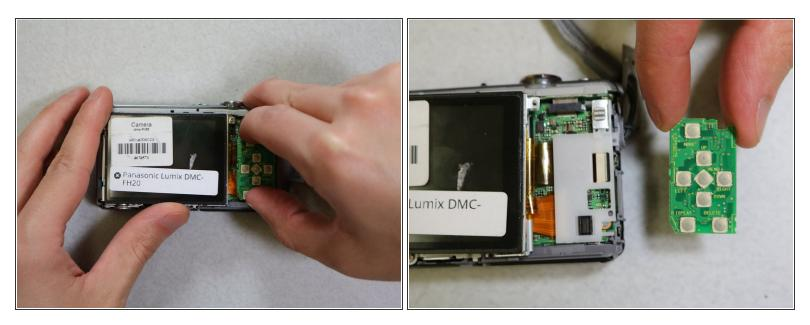
• Remove the circuit board. You should be able to do this with your fingers. Just grab it and pull upwards. If it does not come, use a plastic opening tool to help.
