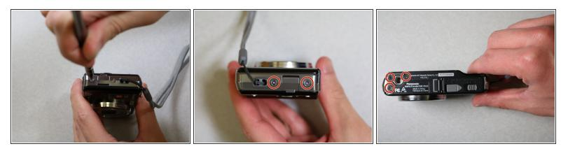
Remove all screws (Phillips #000 head) from the sides and bottom of the camera.
