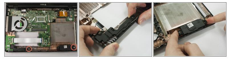
Remove one 3.60mm screw using the ph0 tip from each speaker then lift both up.
