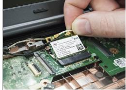
Remove the one 3.85mm screw and remove the WLAN chip.
