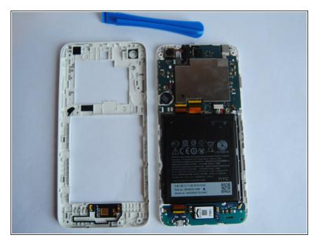
Continue working your way around the seam between the two parts and eventually you will be able to separate the entirety of the backplate revealing the internals of the device.
