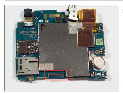
When re-assembling the device. Ensure that the highlighted connector on the back side of the upper logic board assembly is seated properly.
