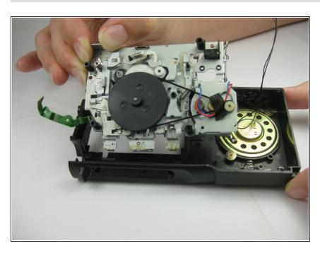
Remove the mechanism deck by lifting the tab as shown.
