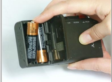
Lift the cover and remove the batteries.
