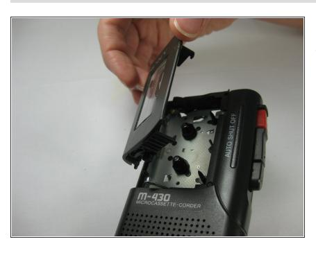
Carefully lift the cassette lid, making sure the tab and latch are free from connection.
