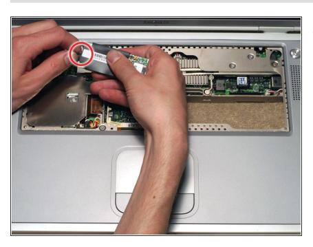
Disconnect the connector cable from the modem.
