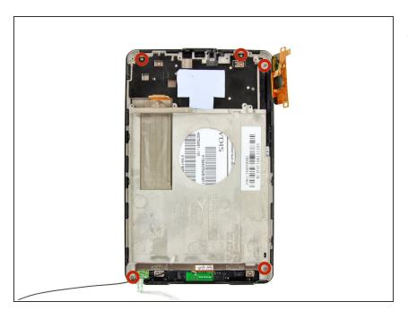
Remove the five 3.6 mm Phillips #00 screws securing the frame and ambient light sensor.
