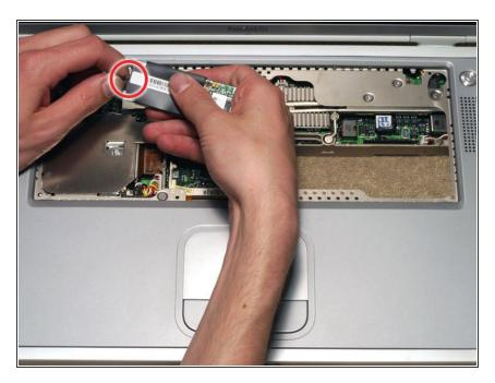
Disconnect the connector cable from the modem.
