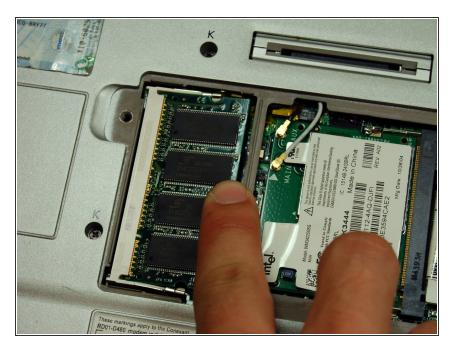
Ensure the memory is in all the way before pressing the memory downward until both metal retainer clips are snapped into place.
