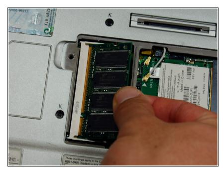
Gently pull the memory out of the retainer at the same 45 degree angle.
