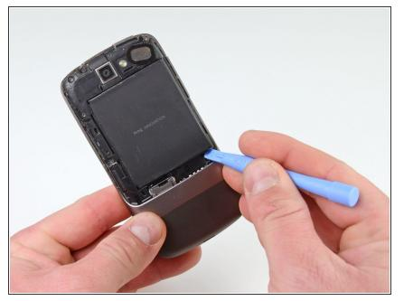
Using the plastic opening tools, pry the left bottom corner of the battery up.
