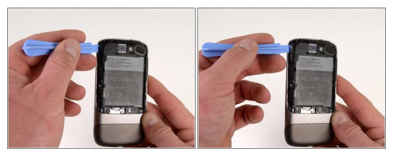
• Pry the upper left tab open on the battery housing.
