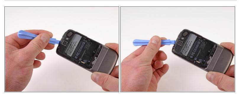
• Pry the top tab of the battery housing.
