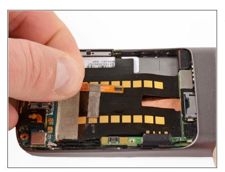
Carefully pull up on the microphone board to release the tape from the phone.
