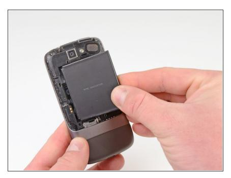
• Pull the battery up and out.
