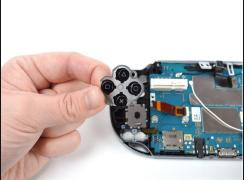
• Using <u>tweezers</u>, gently peel the action button off the back casing assembly.
