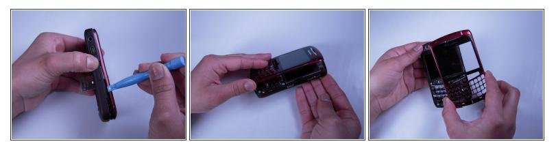
A Be careful not to damage the front cover's plastic clips while trying to separate it from the phone.
