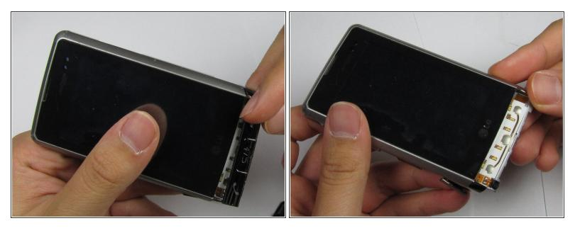
Pry the button panel from the device, starting where the screen and panel connect, until the panel detaches.
