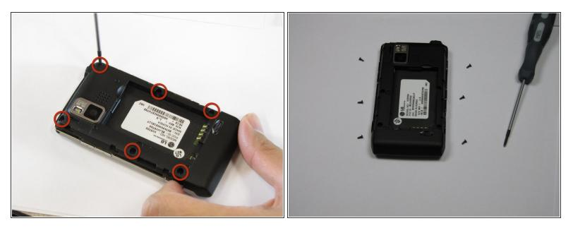
Use the #00 screwdriver to remove the six 4mm phillips screws located around the edges of the phone.
