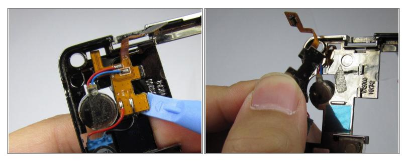
• Using the opening tool, pry the orange connector pad that is securing the earpiece to the frame, away from the device, until it detaches.
