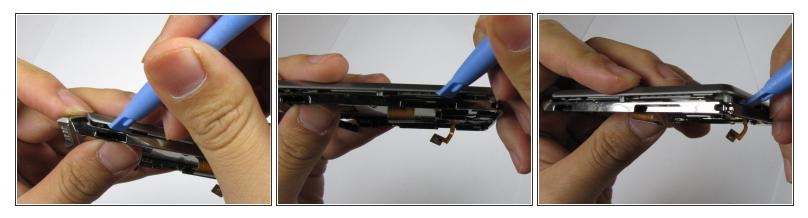
• Using the opening tool, pry the frame from the device, starting at the open edges at the bottom of the device, and working your way around.
