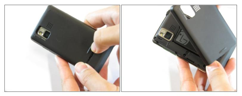
Remove the back cover by firmly pressing against the raised lip on the back panel. Slide the cover towards the top of the phone.
