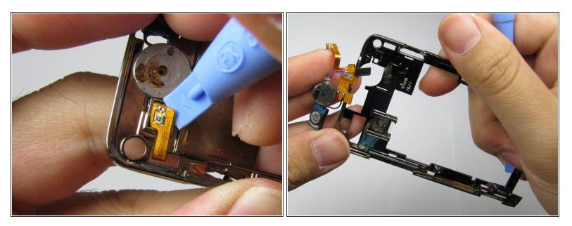
Pry the rest of the orange connector pad --on the opposite side of the device-- away from the frame, and carefully remove the entire earpiece.
