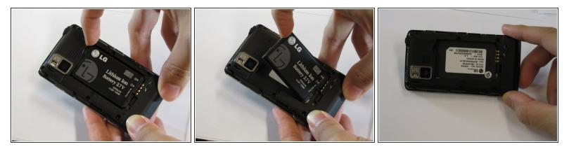
Remove the battery by placing your fingernail or a opening tool in the recessed edge and lift the battery out.
