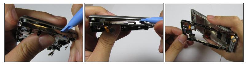
• Gently separate the top of the frame from the back of the device, without completely detaching at the bottom, as shown in the third picture.
