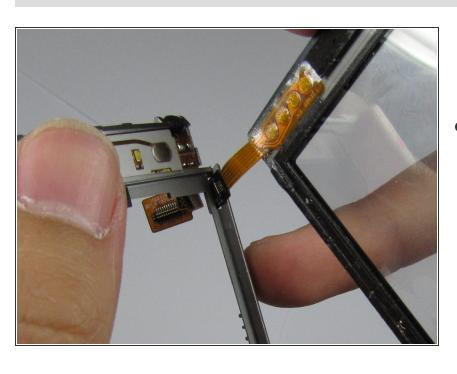
Carefully remove the digitizer connector from the plastic frame.
