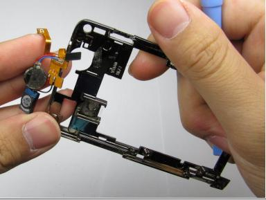
Pry the rest of the orange connector pad --on the opposite side of the device-- away from the frame, and carefully remove the entire earpiece.
