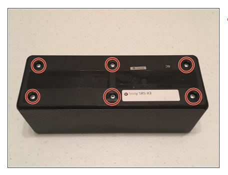
Remove the 6 10mm Philips head screws shown, using a PH1 screwdriver
