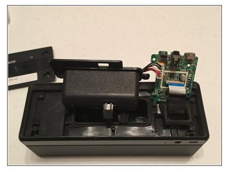
Lift the battery pack and circuit board out of the housing and locate the wires and ribbon connector shown in the figure.
