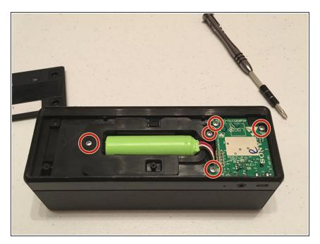
Remove the 5 8mm Philips head screws shown. These are holding the battery and the green circuit board in.
