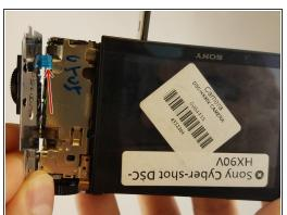
After the outer black panel case of button is removed, gently disconnect the control board data cable to the motherboard utilizing the tweezers gently where the red arrow marks.
