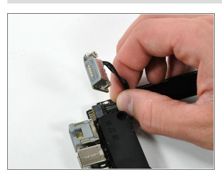
Disconnect the DC-In Board connector from the logic board by pulling it straight away from its socket. To reassemble your device, follow these instructions in reverse order.
