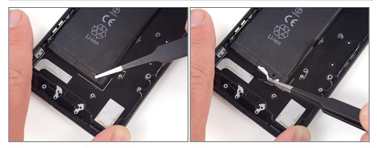
• Use a pair of <u>tweezers</u> with blunt tips to peel back one of the adhesive strips on the lower edge of the battery.
