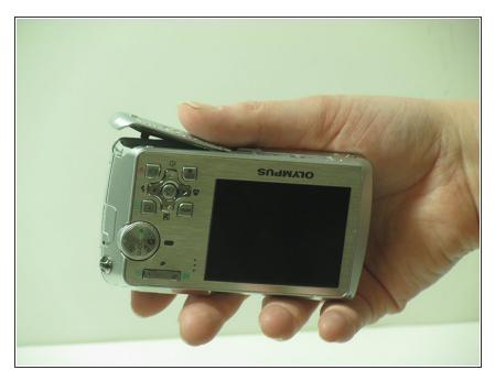
Slide the door located on the bottom of the camera in an outward direction
