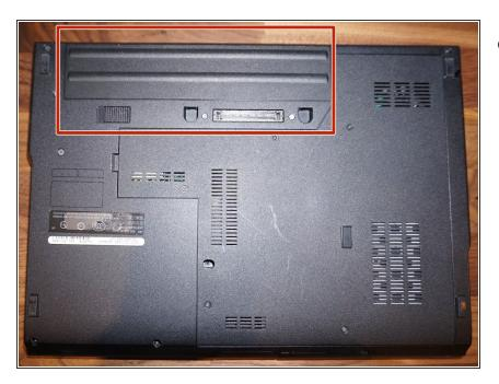
Be sure to remove the battery to prevent any electrical shortage.
