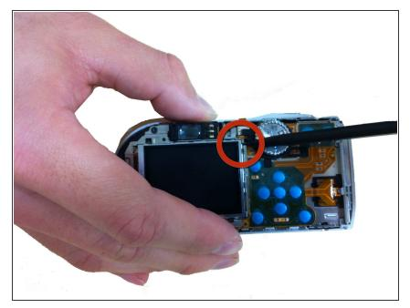
Using a pry tool, gently pry the top right corner of the LCD screen. Pry the screen until the four tabs release it from its current position.
