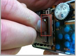
Remove the LCD screen plate by gently pulling upward on the ribbon cable until the screen is removed from the camera.
