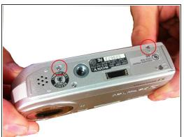
Remove the four screws from the casing.
