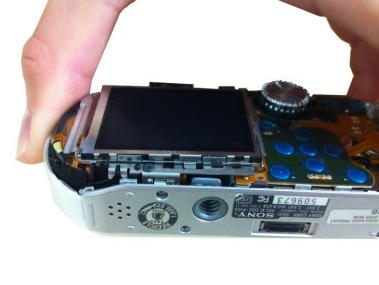
Push the metal tab on the right side of the screen until the plate underneath the LCD screen is released.
