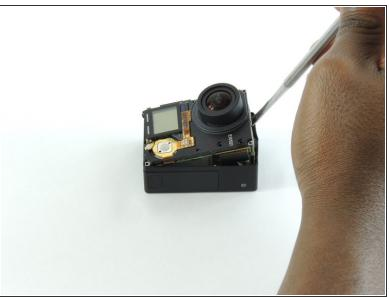
Insert a metal spudger between the back plastic housing and the camera board assembly. Working around the edge to be careful of the inner components, carefully remove the camera.
