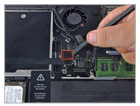
Use the flat end of a spudger to pry the optical drive connector straight up off the logic board.
