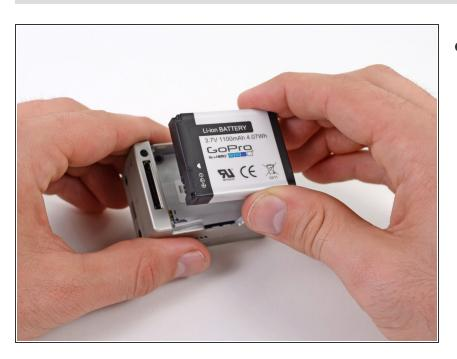
Remove the battery from the case.
