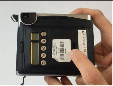
• The battery compartment can be found on the backside of the camera. Pinpoint this compartment and focus on the right edge of the compartment gate to find the opening latch.
