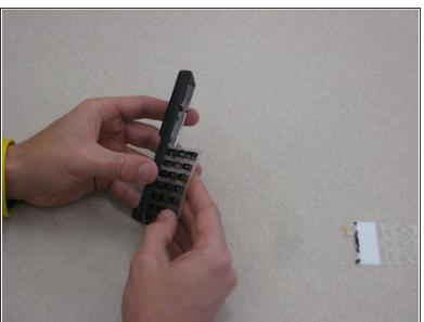
To remove the keypad, tilt the phone and the keypad will slide out with the orientation shown.
