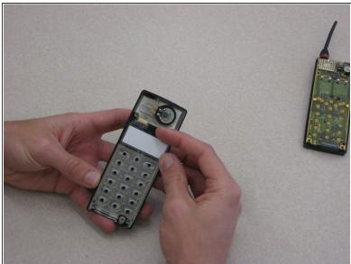
After removing the battery casing and taking apart the phone casing, the keypad is held in with a
