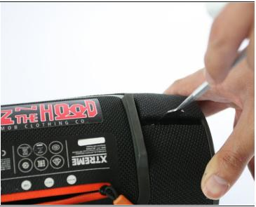
• Use the metal spudger to gently pry and lift the edge of the seam. The cover is held in place with plastic snaps that will make a popping noise when disengaged. !!Start with the back half, this will expose TWO Screws that need to be removed before lifting the front half.
