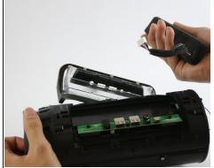
Carefully lift the battery free of the device, threading the cable through the hole in the case as you do so.
