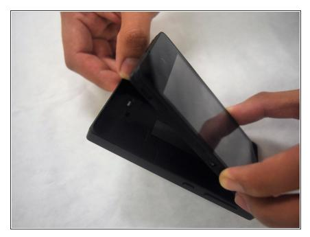
Remove the back cover of the device by applying light pressure toward the outer rim and display.
