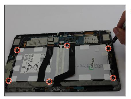
Remove the six 3mm screws around the battery with the <u>Phillips PH000</u> <u>screwdriver</u>.
