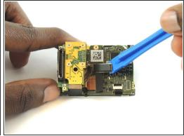
Using a plastic opening tool, separate the camera sensor's connector from the motherboard.
