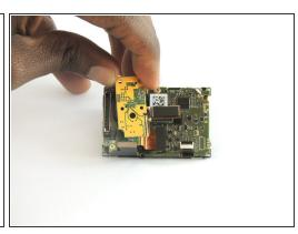
• Using a #00 Phillips head screwdriver, remove the four 3.0mm screws holding the camera sensor.
