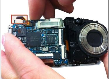
• Using <u>tweezers</u>, gently pull the ribbon trace out of its housing found on the left side of the flash.
