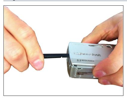
Using a spudger, carefully pry open the front casing.
