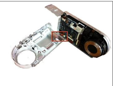
• Carefully separate the front casing from the camera body.
