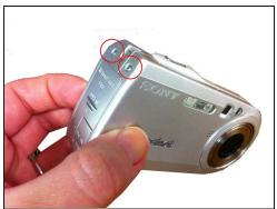
• First locate the appropriate screws for detachment.
