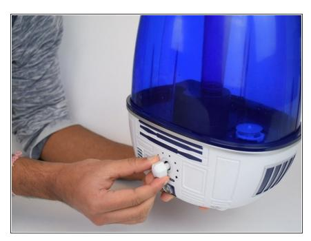
• Remove the dial in the front of the device by pulling the dial outwards.
