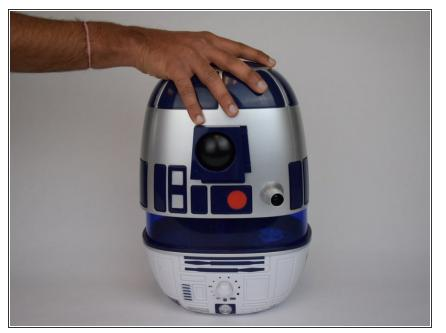
• Remove the top cover by pulling upwards on R2's head.
