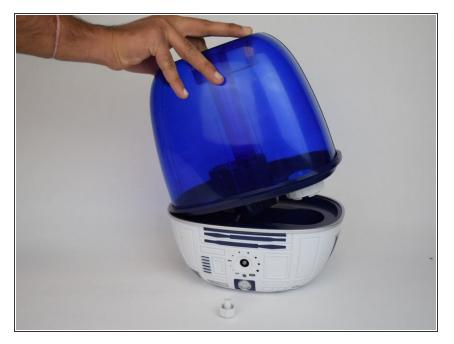
• Remove the water tank by lifting the tank upwards.
