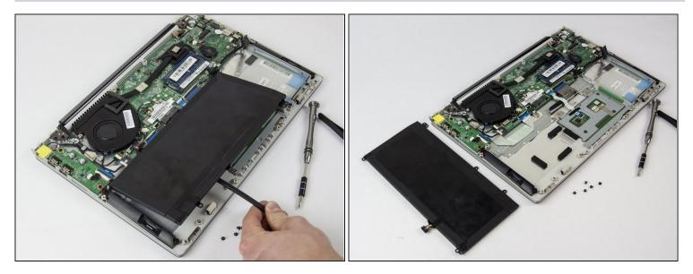
• Once the battery is disconnected, lift up on the front of the battery and remove it from the laptop body.
