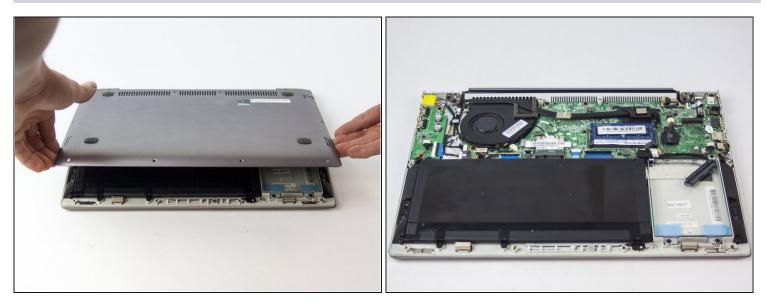
• Starting from the front, use a plastic opening tool to separate the bottom of the case from the body of the laptop.
