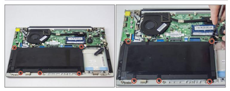
• Remove the five 2.8 mm #1 Phillips head screws that hold down the battery pack.
