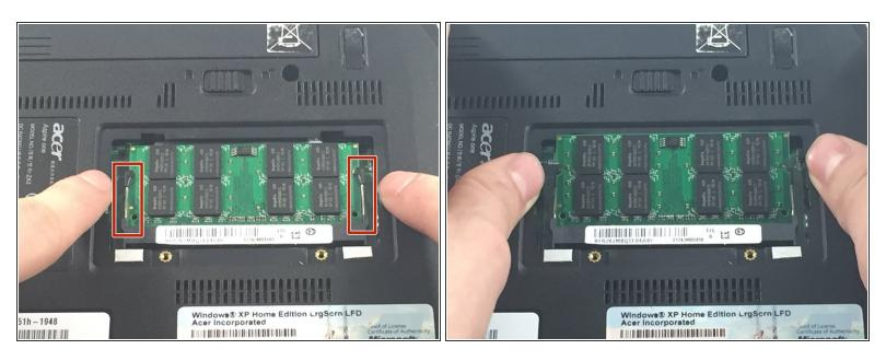
Use your thumbs to push the RAM clips out. The card should lift up when its released. It can then be removed.
