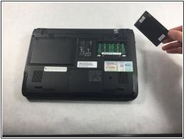
• There are two Phillips #0 (M2-L2.5 mm) screws that is securing the cover. Remove these screws and lift up the cover panel.
