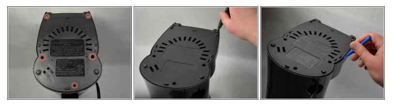
Use a Phillips #1 screwdriver to remove the two 9mm screws and the three 11mm screws on the bottom of the coffee maker and remove the bottom plastic cover.
