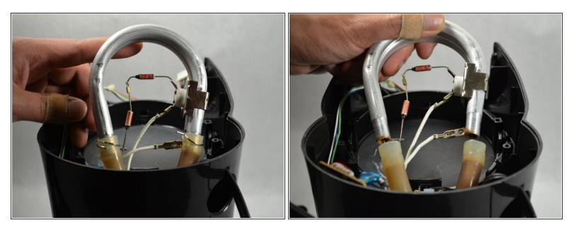
• Remove 2 hose clamps from heating element. Remove heating element from tubes.
