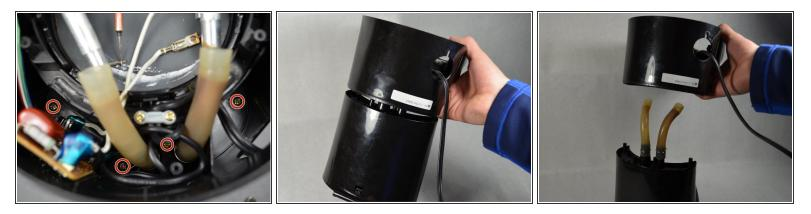
• Using a Phillips #1 screwdriver, remove one 10mm screw, and three 11mm screws connecting the reservoir to the base and remove reservoir from the base.
