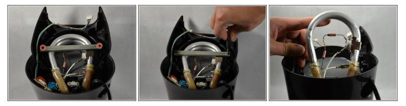
Using a Phillips #1 screwdriver, remove 12mm screws from heating element bracket and remove bracket.
