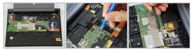
• Before detaching the LCD and digitiser connectors, remove the two small screws at the top left (red bordered area in photo). Remove the metal shield and disconnect the battery wire.
