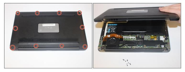
• Remove ten 3mm screws from the back cover with a T5 screwdriver.
