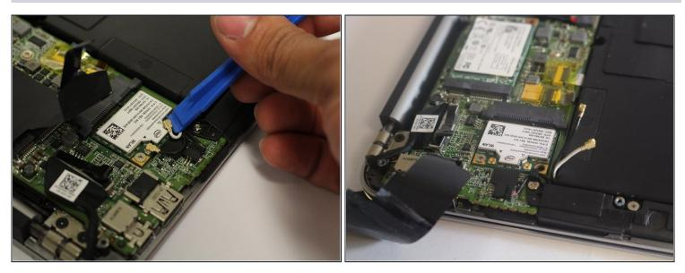
• Use a plastic iFixit opening tool to remove the two wires connected to the wireless card.
