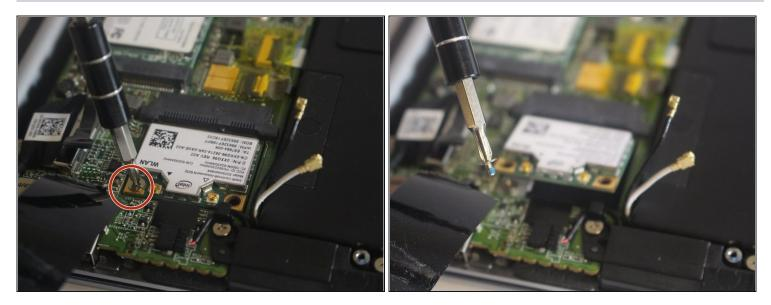
• Use a **PH00** screwdriver to remove the one 3mm screw that holds the wireless card in place.
