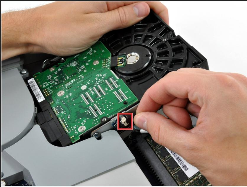
**⚠** The following action is optional. If you skip this step, be very careful not to strain the thermal sensor cable as you disconnect the hard drive cables and transfer this bracket to your new hard drive.
