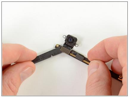
• Using the flat end of a spudger, pry the rear facing camera off of its socket on the underside of the headphone jack assembly board.
