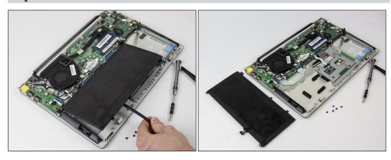
• Once the battery is disconnected, lift up on the front of the battery and remove it from the laptop body.
