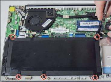
• Remove the five 2.8 mm #1 Phillips head screws that hold down the battery pack.
