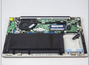
• Starting from the front, use a plastic opening tool to separate the bottom of the case from the body of the laptop.
