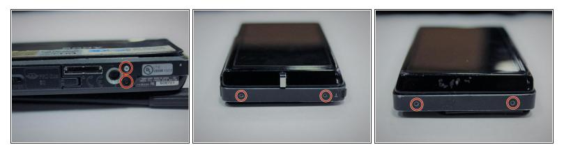
• Use a Phillips #0 screwdriver to unscrew the six 2mm screws on the outer case of the camera.
