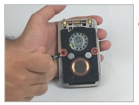
Remove the two Phillips PH0 (0.9mm) screws located to the side of each magnet.
