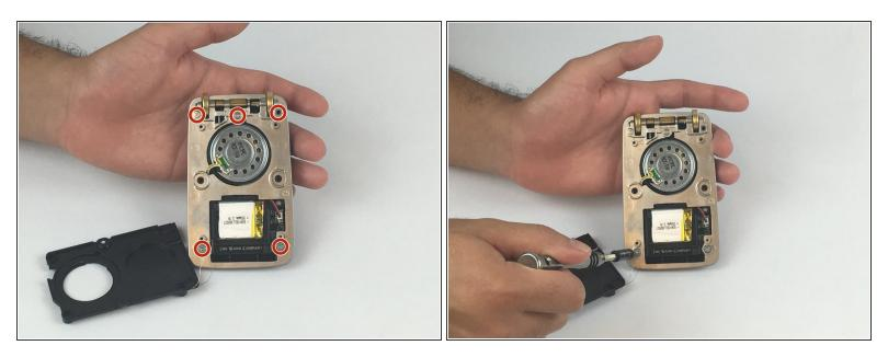
• Remove the five Phillips PH0 (0.9mm) screws located at the top and bottom of the silver plate.
