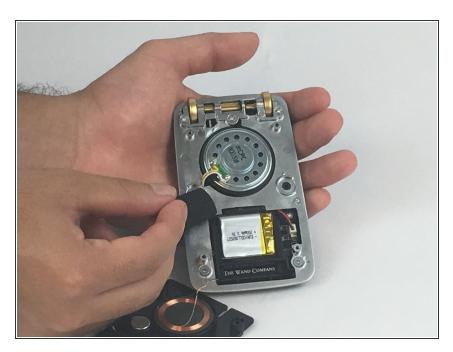
• Remove the protective foam attached to the battery.
