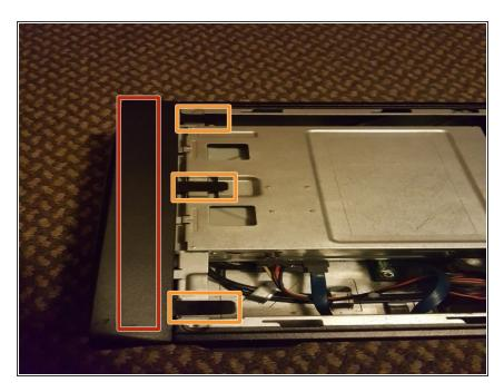
While putting LIGHT downward pressure on the side of the face cover (red), apply gentle upwards pressure to the three clips (Orange).
