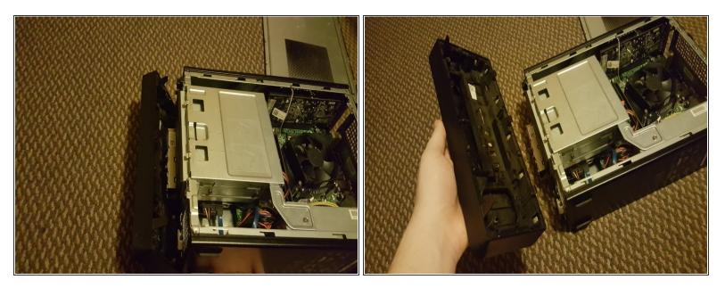
• Once the three clips are free from the internal case you will see the face panel swing down. Simply lift the front of the PC up while it is laying on it's side, and the face cover will unhook from the other side.
