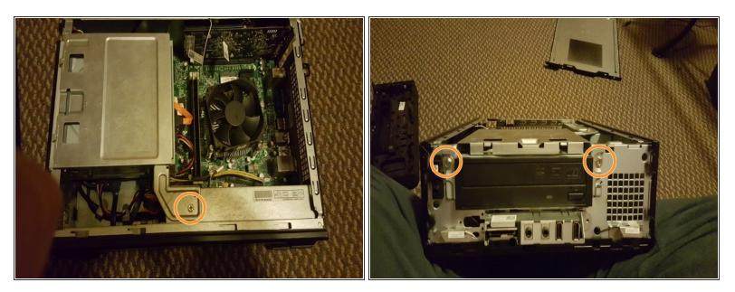
Next remove the three screws holding the HDD and Optical Drive in place. It is very important that you **DO NOT** remove the drives yet as they are still plugged into the motherboard.
