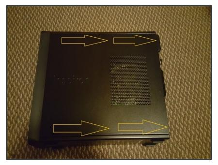
Next we are going to lay the tower on it's right side (side where motherboard is attached) and slide the cover off.
