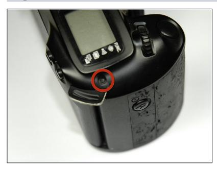
Using a #00 Phillips screw driver, unscrew the one 5.7 mm Phillips screw located next to the LCD screen.
