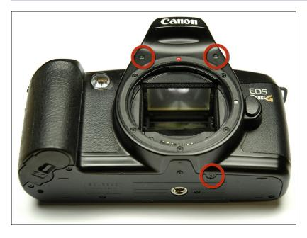
Using a #00 Phillips screw driver, remove three 4.4 mm Phillips screws as indicated by the red circles.
