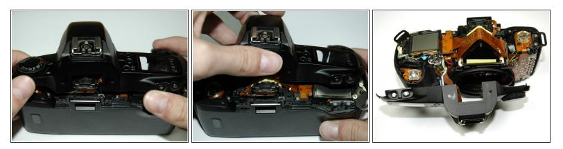
• Remove the top panel by lifting it from the back, pushing it forward over the camera and letting it rotate down in front of the camera.
