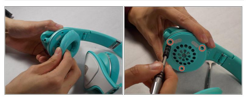
Remove the ear cushions and use a Phillips #2 screwdriver to unscrew the three 5mm screws.
