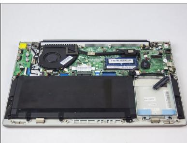
Starting from the front, use a plastic opening tool to separate the bottom of the case from the body of the laptop.
