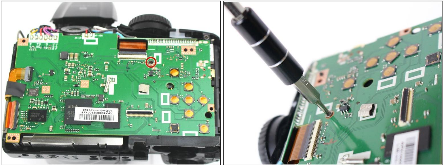
**⚠** When removing the screw attached to the motherboard, proceed slowly and apply only light pressure.
